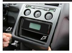
Unclip and remove OEM panel (see arrows)
