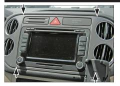
Unclip and remove OEM panel (see arrows)
