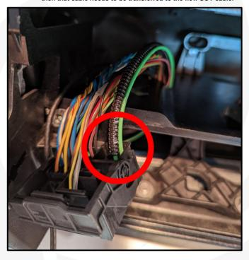
7. Loosen the connector with a small flat head screwdriver
