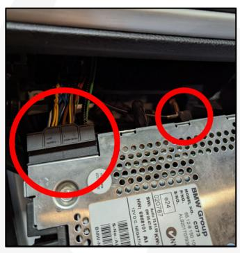
6. OBS! If there is a fiber optic cable in the OEM connector, then that cable needs to be transferred to the new SOT cable.
