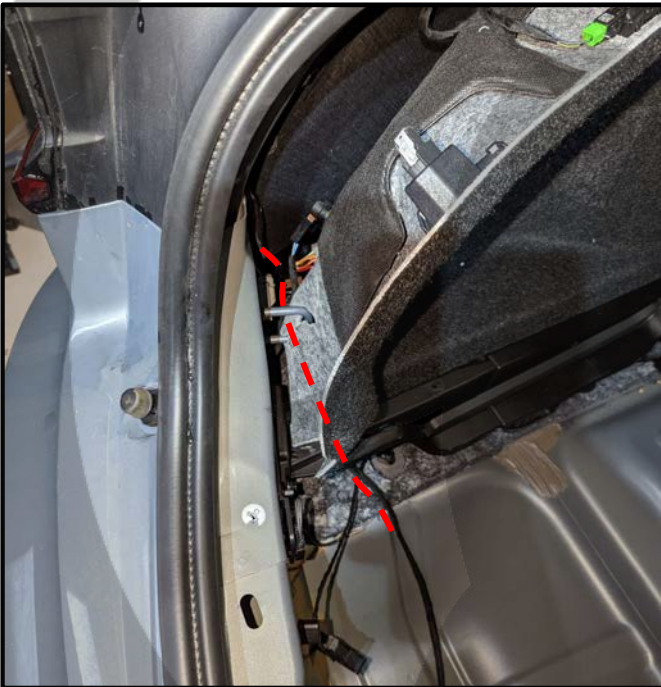
13. Route SOT cable under the panel
