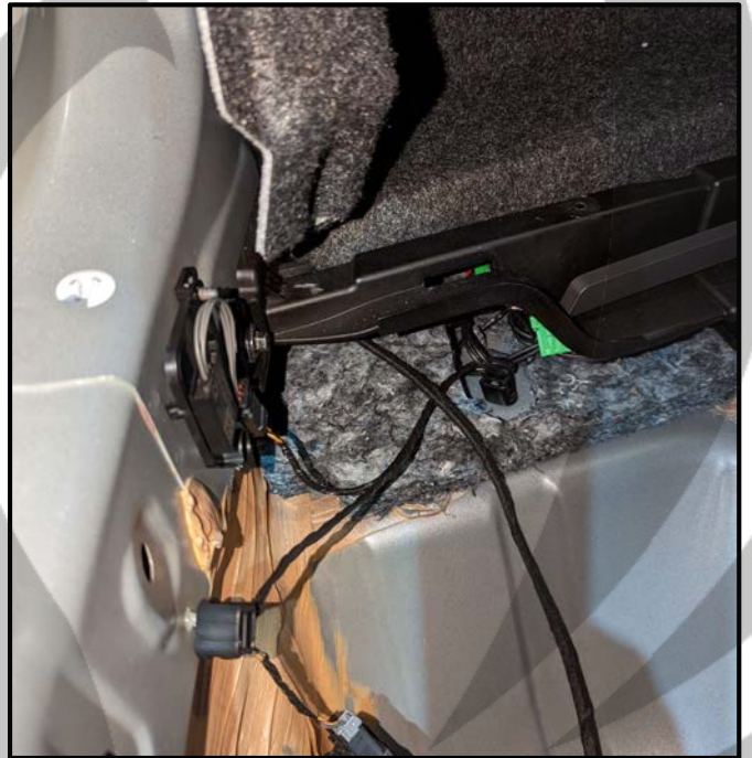
14. Cable routed under the panel
