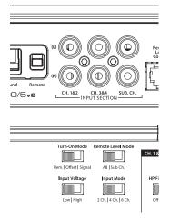
If you wish to send six discrete channels into the XD700/5v2, simply use all six inputs and set the "**Input Mode**" switch in the "**6 Ch**." position. The amplifier will automatically combine the left and right "**Sub Ch**." input signals to mono. If you have only one channel of subwoofer signal available, it is acceptable to only use one of the "**Sub Ch**." inputs, but for optimal gain, we recommend using a Y-adaptor and feeding both "**Sub Ch**." inputs.
