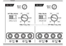
"Filter Mode" Controls: The XD700/5v2 employs 12dB per octave filters for each pair of main channels (one high-pass filter for channels 1&2 and another high-pass / bandpass filter for channels 3&4. The subwoofer channel provides a low-pass filter with the option of 12dB or 24dB / octave slopes. Each of these filters can be controlled or defeated completely by way of the three-position "Filter Mode" switches in each channel section:
