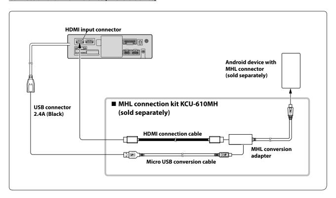
• A connection kit or adapter kit suitable for the type of terminal on the connecting device is required.
