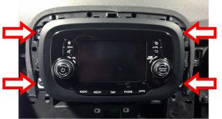
Remove four highlighted screws and remove the OEM head unit.
