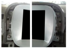
Fit Brackets to aftermarket radio and fit radio into the dashboard.
