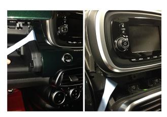
Remove the plastic panel from below the radio using a panel removal tool.
